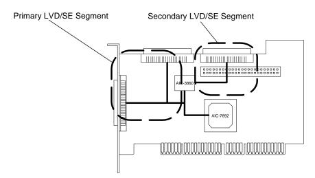
Figure 1-2. Primary and Secondary Bus Segments
